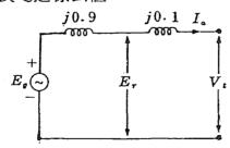
$jx_* = j\ 0.1$  標么  $jx_* = j\ 1.0$  標么  $V_* = 1.0$   $\left\lfloor 0^\circ \right\rfloor$  標么  $jx_* = j\ (x_* - x_*) = j\ 0.9$  標么  $I_* = 1.0$   $\left\lfloor -30^\circ \right\rfloor$  標么  $(a)E_* = jx_*, I_* = j\ 0.9 \times 1.0$   $\left\lfloor -30^\circ \right\rfloor = 0.9$   $\left\lfloor 60^\circ \right\rfloor$  標么  $(b)E_* = V_* + j\ (x_* + x_*, )\ I_* = V_* + jx_*, I_* = 1.0$   $\left\lfloor 0^\circ + 1.0 \right\rfloor = 1.0$
